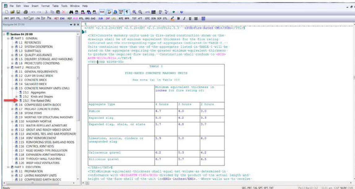
The screenshot shows a software application window with a project tree on the left and a table in the main window. The project tree is expanded to show 'Section 04 20 00' and 'PART 2 PRODUCTS', with '2.5 CONCRETE MASONRY UNITS (CMU)' selected. The table in the main window is titled 'TABLE I FIRE-RATED CONCRETE MASONRY UNITS' and lists various aggregate types with their minimum equivalent thicknesses for 4, 3, and 2 hours of fire rating.
